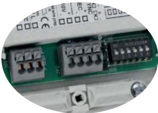
Terminals and dip-switch selection
