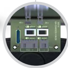
Integral switches for multi-wattage and selectable CCT options
